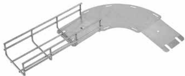
2. Attach first tray with washer support and 1/4\"-20 nut and bolt
