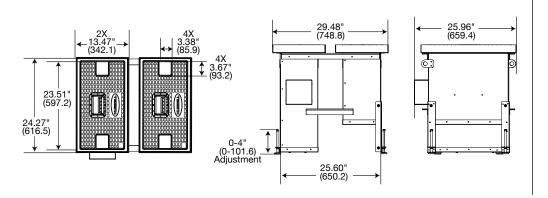
Stand Alone Water/Air Box HBLSCCUBW (Painted Galvanized) HBLSCCUBWSS (Stainless Steel)
