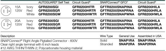
SNAPConnect GFCI must use a SNAPConnect Pigtailed connector.
