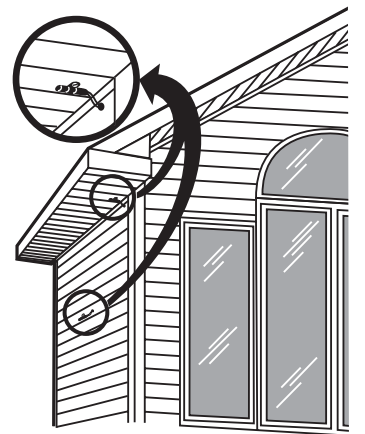
Fig. 7. Outdoor temperature sensor installation.
