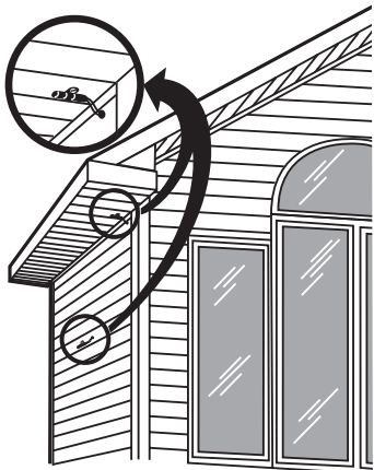
Fig. 7. Outdoor temperature sensor installation.
