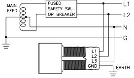
(L1-L3, GND) See Wire Identification Diagram
