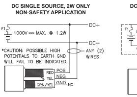
**R-3D2 WIRING CONFIGURATIONS**
