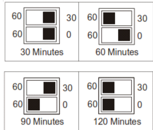
Dipswitch Settings for Selection of Defrost Time
