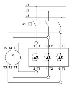
**Note:** For soft starters used in an Inside-the-Delta application, use of a shunt trip breaker is highly recommended. The S811+ may be configured to actuate a shunt trip breaker on user selected Fault Trip parameters.
