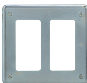
For GFI receptacles; rectangular height 2\frac{5}{8} "; rectangular width 1\frac{5}{16} "
