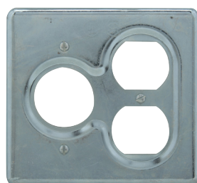
For round flush receptacles (hole diameter 1\frac{13}{32} ""); duplex convenience receptacles, standard and 2-wire, 3-pole grounding (hole diameter 1\frac{11}{32} "")
