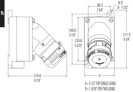
OConsists of: EDS(C) back box as applicable; ENR5151 M4 or ENR5201 M4 as applicable; GFS1 M4.
