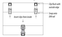
3. To prevent horizontal shifting across the DIN rail, use two Eaton IQ35M-DRSC end stop clips or equivalent.
