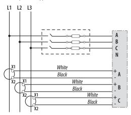
Diagram 5: 3-Phase 4-Wire Wye Direct Voltage Connection 3 CT
