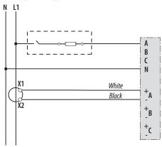
**Diagram 2: 1-Phase Line-to-Line 2-Wire System 1 CT**Use System Type 11 (2L)
