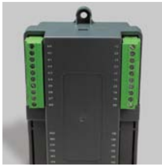
I/O Expansion Modules available in 8-in/6-out and 16-in/12-out.
