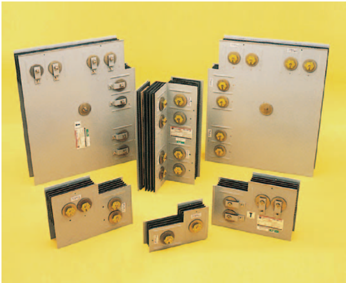
Corner Joints The exclusive Pow-R-Way III corner joint elbow can solve any difficult pathway problem with leg lengths as small as 4.71 inches (119.6 mm) for an upward or 4.35 inches (110.5 mm) for a downward elbow. The corner joint is provided with torque-indicating bolts, fall-away instruction tags, and the heavy-duty captive nut retainer. The photograph depicts a 1000A (front foreground), two 2500A (foreground), a 5000A upward (center background) and two 5000A forward.
