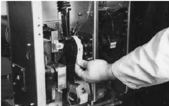
Figure 6-16 Remove Marked Masking Tape From Cam
