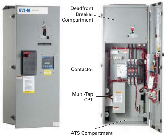
40-200 A Service Entrance Contactor NEMA 1
