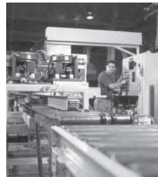
Final Busway Assembly
