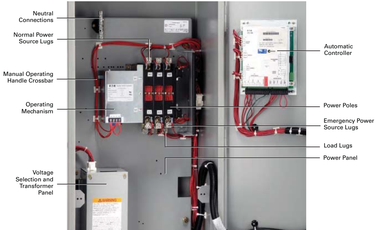
Typical Contactor-Based ATS 100–400 A
