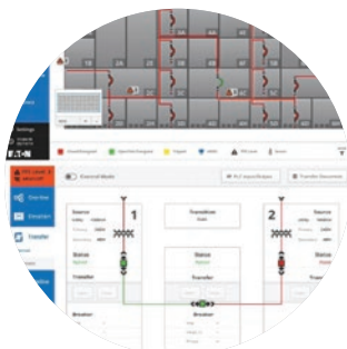
Low voltage switchgear elevation and one line view
