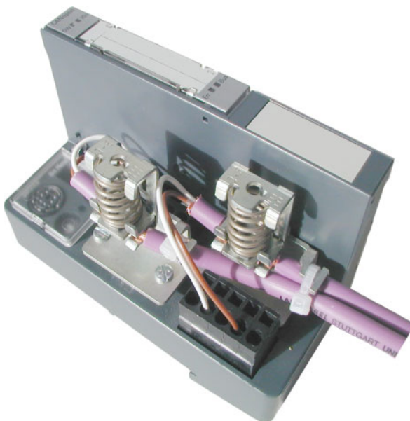
Figure 7: Shielding connection for an XN-GW-CANopen
