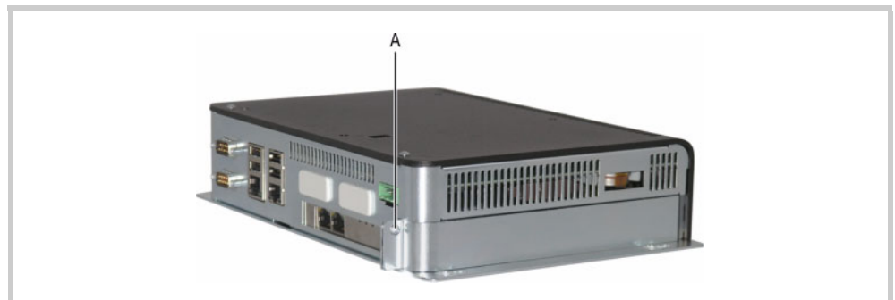
Fig. 25 Fastening the PCI expansion card and the side cover
