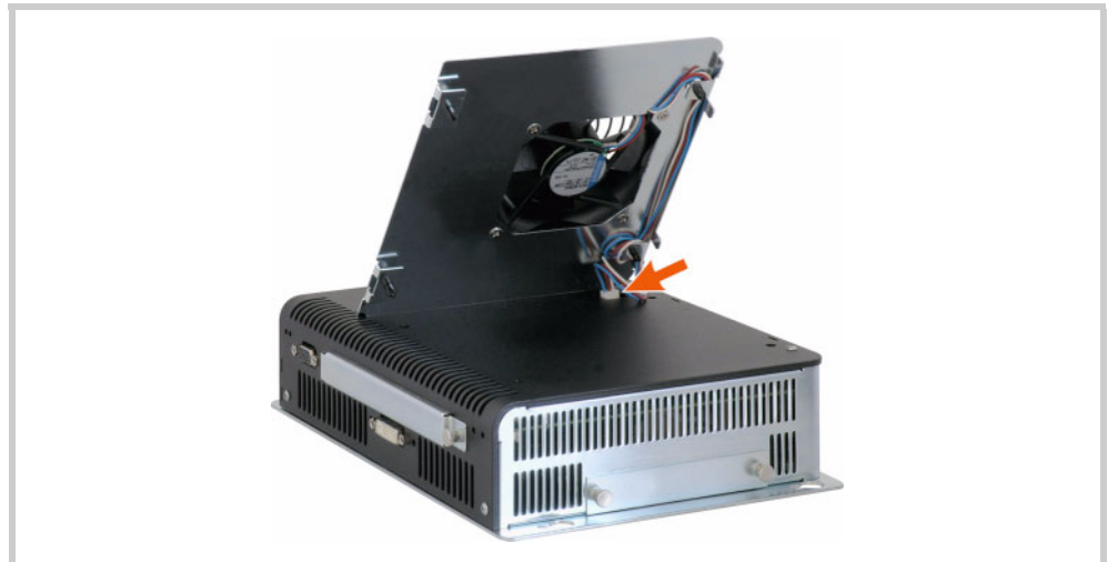
Fig. 48 Connector for the power supply of the active cooling unit
