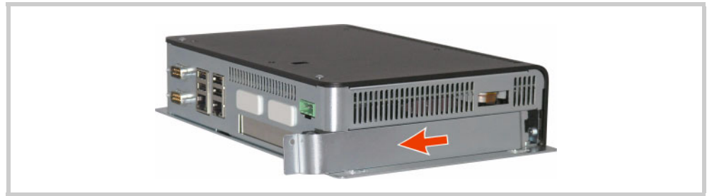
Fig. 21 Removing the side cover
