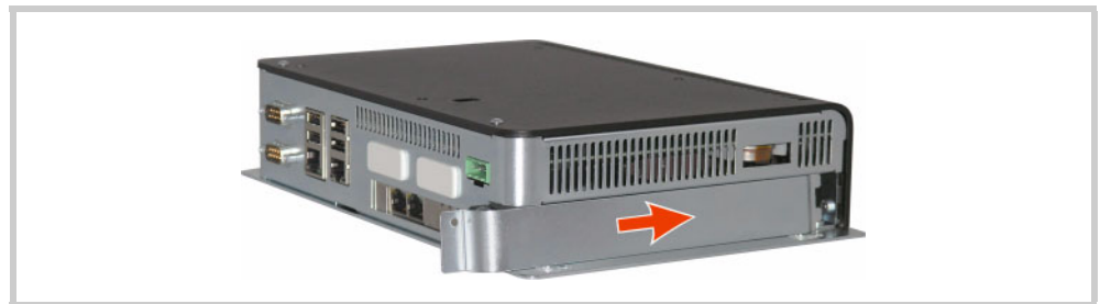
Fig. 24 Positioning the side cover
