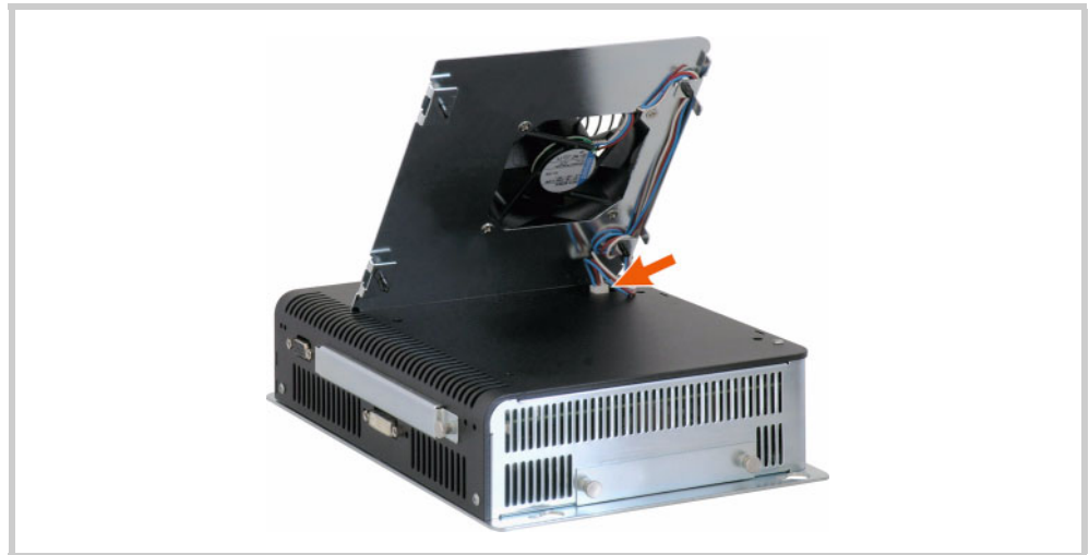
Fig. 30 Power supply for the active cooling unit connected
