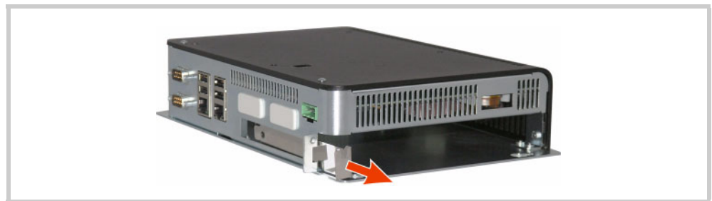
Fig. 22 Removing the PCI card slot cover
