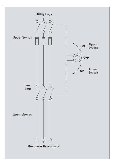
Double-Throw Switches Have Two Interlocked Switches with a Common Load Side Connection
