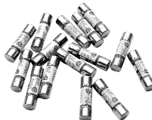
Fuses, dual element miniature type, 500-Volt 1 1/2 in. long, 13/32 in. dia. for use with Style No. 2147A15G15 or G16 1 Amp Qty. 5 10 Amp Qty. 5 15 Amp Qty. 5
