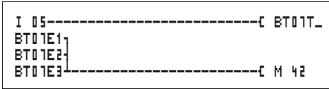
Figure 99: EZD circuit diagram with enabling of transfer data block function block
