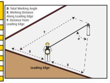
For example, if the anchorage connector is 6' from the leading edge (Y), the working distance (X) is 8' in each direction from the perpendicular, which translates to a 53° working angle.
