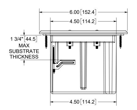
1.) BOX MATERIAL: POLYCARBONATE, COVER PLATE MATERIAL: NICKLE PLATED BRASS, COVER MOUNTING SCREW MATERIALS: NICKLE PLATED BRASS, DEVICE MOUNTING SCREW MATERIALS: ZINC PLATED STEEL, FLANGE MOUNTING SCREW MATERIALS: BLACK PHOSPHATE COATED STEEL WING MATERIAL: ZINC PLATED STEEL, GROUND PLATE MATERIAL: ZINC PLATED STEEL, GASKET MATERIALS: DOLYTIPETHANE FOAM MATERIALS: POLYURETHANE FOAM 2.) UL LISTED, FLOOR BOX MEETS UL514C SCRUB WATER EXCLUSION TEST
