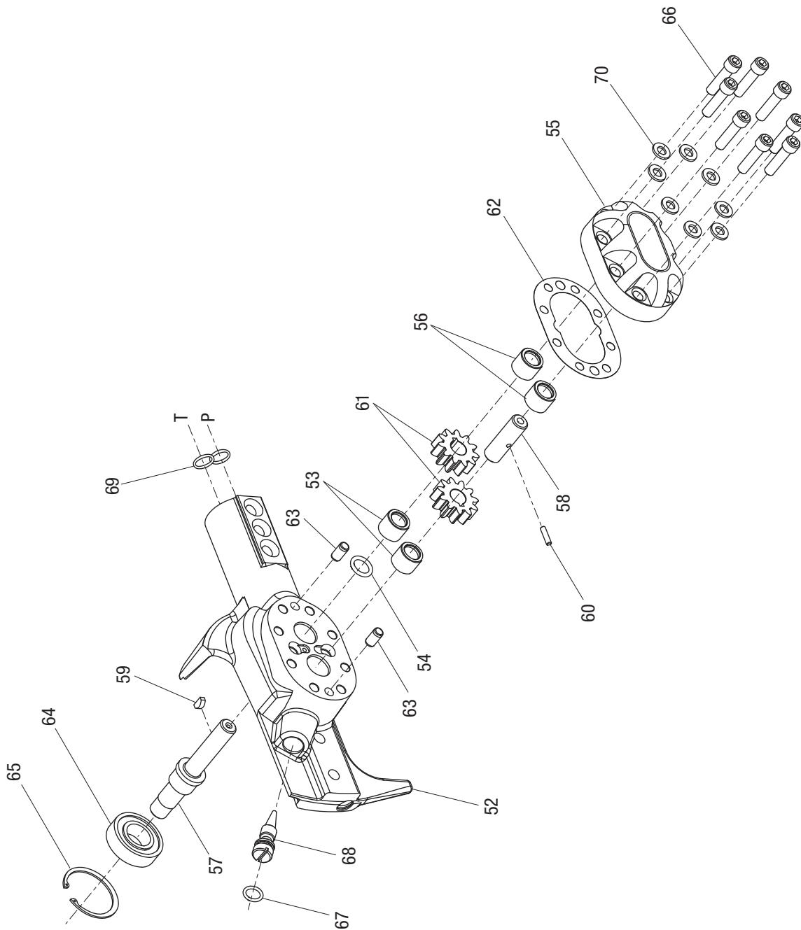
**Illustration—Motor Assembly for Serial Codes FRM, FRP, and FRR**
