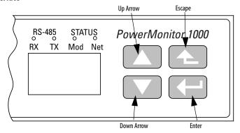
The buttons function differently in each mode. The power monitor enters into Display mode by default.
