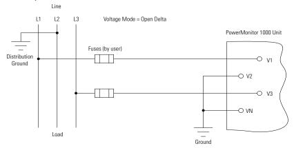
Maximum line to line voltage 347V. If line to line voltage exceeds 347V, then PTs must be used.
