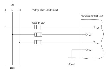
Maximum line to ground voltage is 347V. If line to ground voltage exceeds 347V, then potential transformers must be used. The unit indicates voltage overrange (999.0) if an intentional or accidental ground causes line to ground voltage in excess of 347V.
