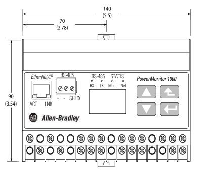
All dimensions are mm (in.). Panel mount depth 59 mm (2.4 in.). DIN-rail mount depth 62 mm (2.44 in.). Hole spacing tolerance:  $\pm 0.4$  mm (0.016 in.).
