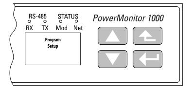
When the correct password is entered, Program Setup appears in the display. The power monitor is now in Program mode.
