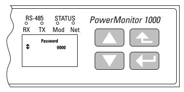
**4.** Press <enter> if the password has not been changed from the default (0000). If the password has been changed, then enter the correct password.
