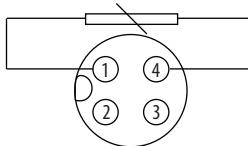
The screw-in thermometers of the 837RTD are built in two-wire connections. The resistance of the connecting leads affects the measurement value of two-wire connections and must be considered. For copper cable with cross section 0.25 mm<sup>2</sup> (24 AWG), the following value applies: 0.163 Ω/m 0.04° C/M for PT 1000 and 0.4° C/M for PT 100.
