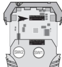
Set upper measurement frequency via the DIP switches S1 and S2.1, S2.2 (see table).
