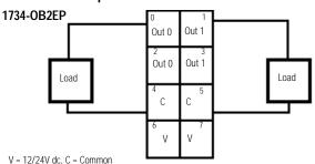
Field power is supplied from internal power bus
