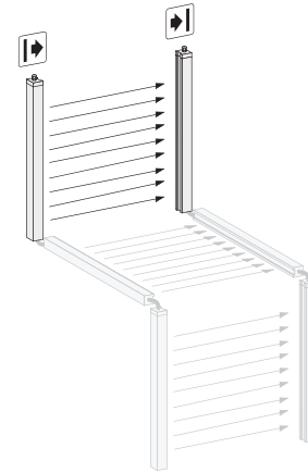
Up to three GuardShield POC segments can be interconnected.
