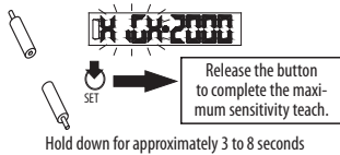
Figure 13 - Maximum Sensitivity with Percent Indication
