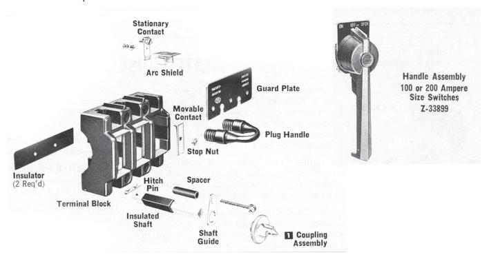
Coupling Assembly is included in the Handle Assembly repair part number Z-33899.
