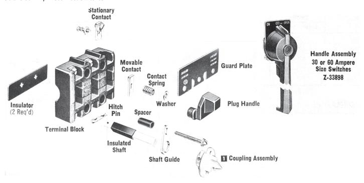
Coupling Assembly is included with the Handle Assembly repair part number Z-33898.
