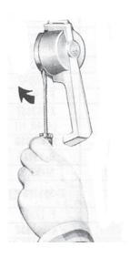
When moved to the "Off" position, the spring-driven mechanism "snaps" open the moveable contacts in a "quick break" action. The enclosure door remains interlocked to the disconnect switch until the handle is moved to the "Open" position. Handle assemblies are designed to accommodate padlocking in the "Off" position.
