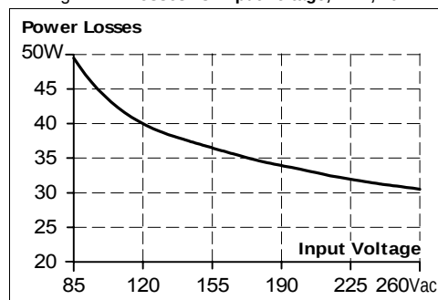
Fig. 11-4 Losses vs. input voltage, 24V, 20A
