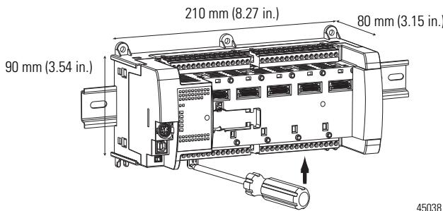
Mounting dimensions do not include mounting feet or DIN rail latches.
