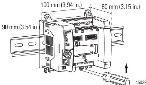
Mounting dimensions do not include mounting feet or DIN rail latches.
