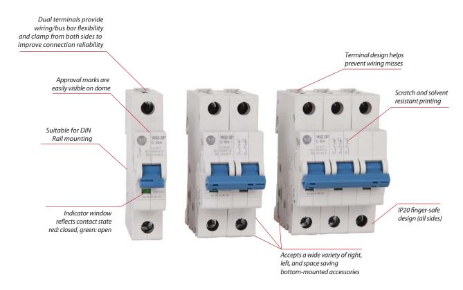
Bulletin 1492-SP thermal magnetic Supplementary Protectors provide overcurrent protection for equipment where branch circuit protection is already provided, or is not required. These devices are also Miniature Circuit Breakers as defined by IEC Standards.
