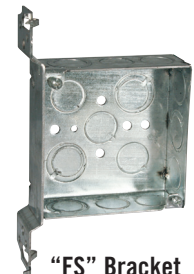
"FS" Bracket Mounts on flat side of stud. Gauging tabs and recessed nailing spurs.
