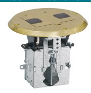
Wood floor boxes allow for the placement of electrical power or a combination of power and voice/data devices. Boxes easily mount into the floor and are height adjustable (up to inch) for optimal alignment and fit.
